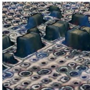
Systems for an objective three-dimensional reconstruction of the surface of samples with an equitable metrological evaluation of the third dimension are an important tool in the characterization of the quality of surfaces such as roughness, porosity etc. In addition to giving complete information of the shape, it also allows objective measurements: volume, depth, tool wear, and comparison of shapes.
