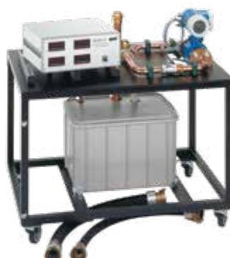
**HM 332****Pump characteristics for parallel and series configuration**
