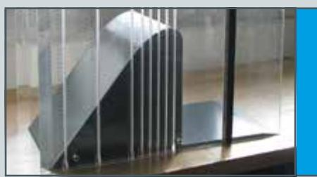
HM 162.34 Ogee-crested weir with pressure measurement
