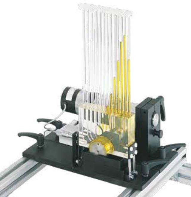
**TM 260.05****Dynamic friction in cylindrical pin – roller**
