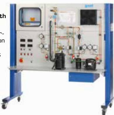
**ET 380****Refrigeration cycle: refrigeration plant and heat pump**
