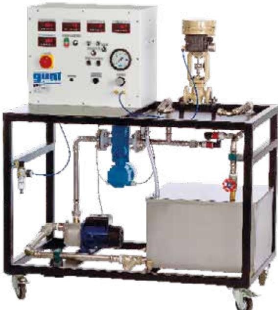
**RT 395****Maintenance of valves and fittings and actuators**
