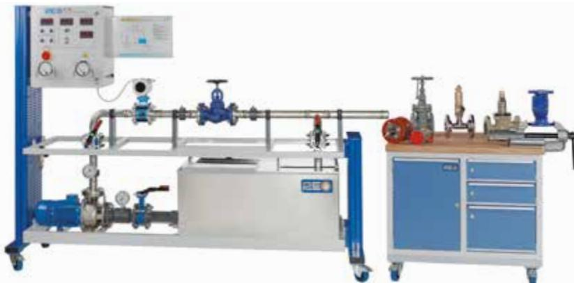
**RT 390****Test stand for control valves**
