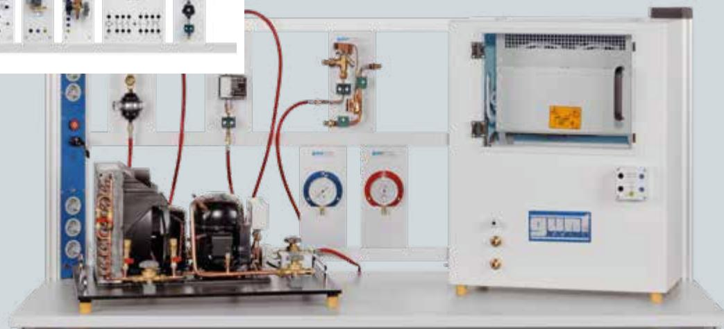
Experimental setup capacity control with post injection with ET 910, ET 910.10 and ET 910.11
