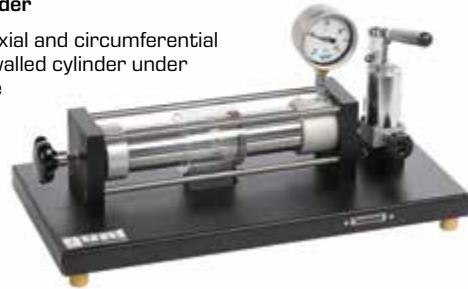
**FL 140****Stress and strain analysis on a thick-walled cylinder**
