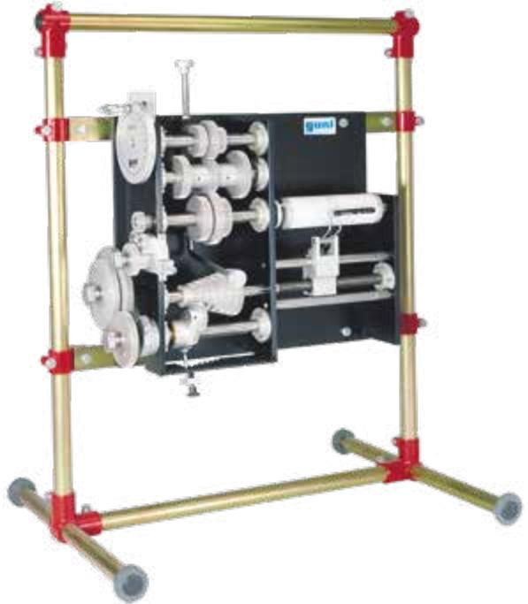
**AT 200****Determination of gear efficiency**
