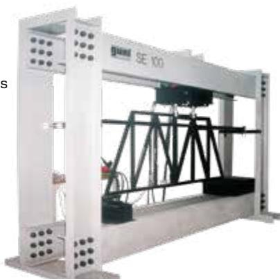
**SE 110.48****Bending test, plastic deformation**
