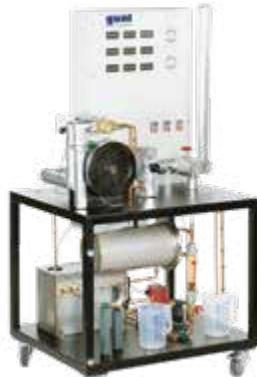
Experimental plant with two-cylinder steam engine ET 813, steam generator ET 813.01 and brake unit HM 365
