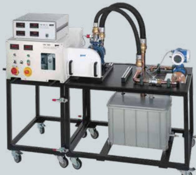
Trainer for centrifugal pumps with supply unit HM 365.10, centrifugal pump HM 365.11 and drive unit HM 365
