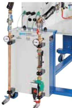
**ET 352****Vapour jet compressor in refrigeration**
