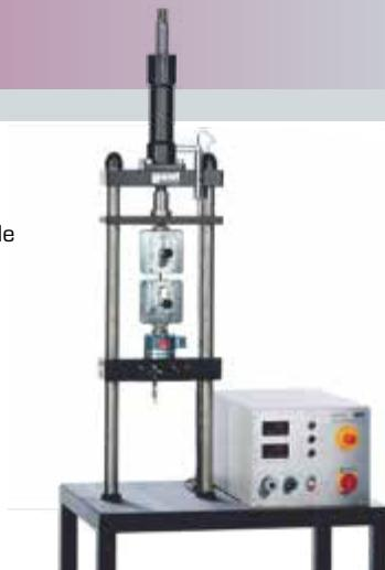
**SE 100****Frame for load testing, 400 kN**
