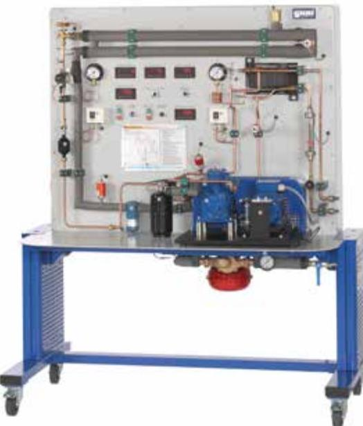
**ET 351C****Thermodynamics of the refrigeration circuit**
