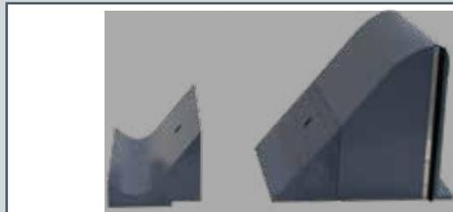
HM 162.32 Ogee-crested weir with two weir outlets
