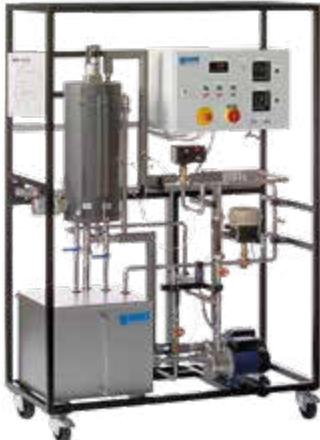
**RT 681****Multivariable control: vacuum degassing**
