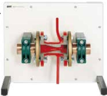
**HM 700.04**Cutaway model:
