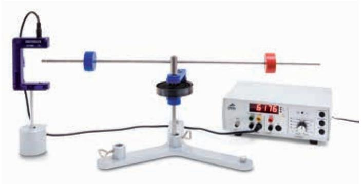
**Moment of inertia  $J$  of weights as a function of their radius  $r$  from the axis of rotation**
