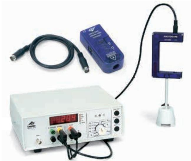
*For measuring times when, e.g. a swinging pendulum obscures a sensor*
