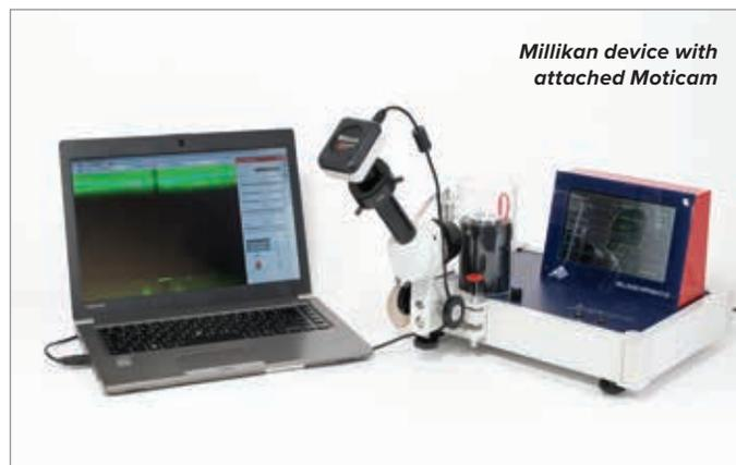
*Millikan device with attached Moticam*
