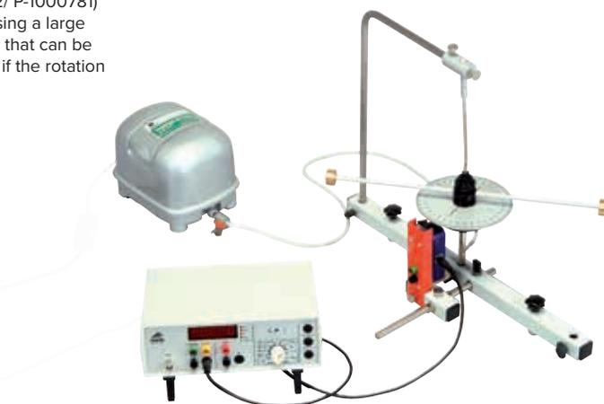
Measuring the period of oscillation and determining the moment of inertia
