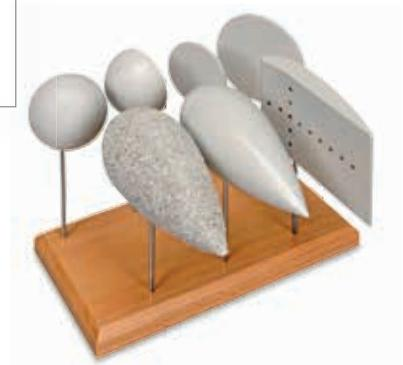
**Set of bodies for air resistance and buoyancy experiments**
