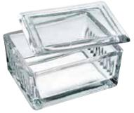
Schiefferdecker Staining Dish For 20 slides 76x26 mm<sup>2</sup> (back to back), with cover. B-1008920
